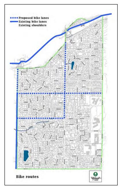
Figure 6.9: Clyde Hill's Bike Routes. Solid blue lines indicate existing bike lanes and shoulders. Dotted blue lines indicate proposed bike lanes.
